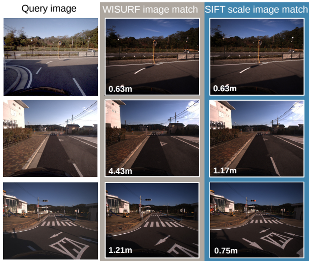
Figure 5. Example image matching results of query images (left) using the WISURF image descriptor (center) and SIFT feature scale (right). Current localization errors are shown in the bottom left-hand corner.
