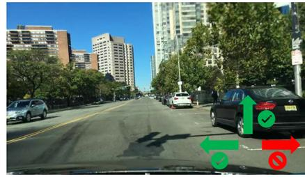
Fig. 3. Typical scene in the BDD-3AA dataset. As shown in the above image, there is a vehicle on the right, thus the steering right action is not available; there are vacant spaces in the front and left, thus the acceleration and steering left actions are available. In the bottom right of this image, the red arrow indicates the corresponding driving action is unavailable, the green arrow indicates the corresponding driving action is available.
