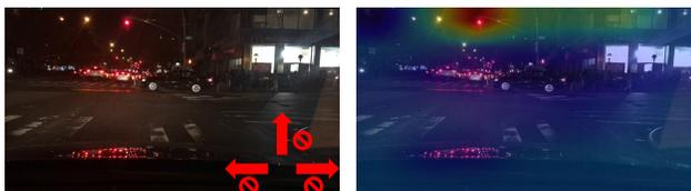
Fig. 7. There are SOB's predictions and explanations for the red traffic light driving scenes. The left image is the prediction results, and the right one is the corresponding explanations. We can see that not only the prediction result is correct but the attention of the SOB is also focused on the red traffic light.
